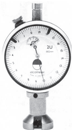
Figure 13.12 Roughness gauge of the type Elcometer 123
