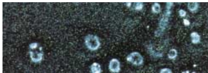
FIGURE 28-6 Fish-eyes can form when painting a silicone or oil contaminated surface. Paint additives can help correct fish-eye problems if sprayed again before full flashing.
