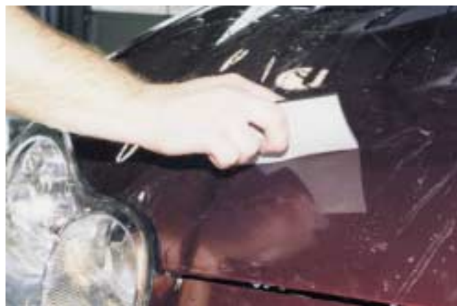
FIGURE 28-22 When wet sanding, squeegee off the water so you can see if the flaw has been leveled. (Photo courtesy of Norton)
