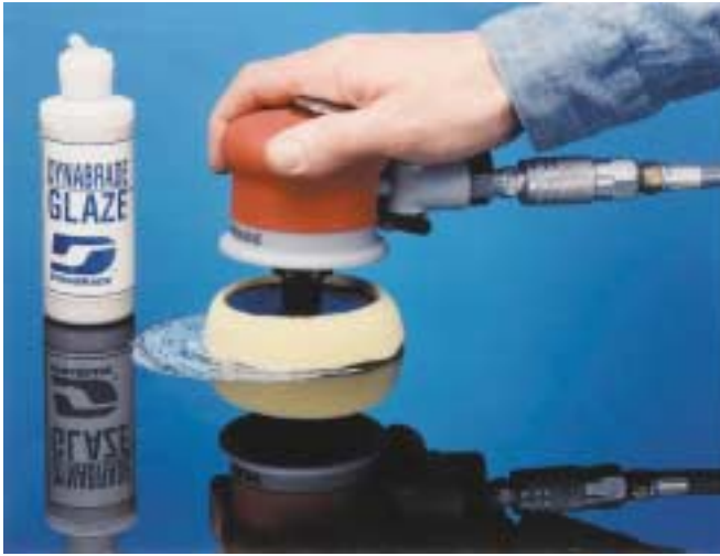
FIGURE 28-25 Compounding removes a thin layer of paint and is needed to return the paint gloss after wet sanding. (Dynabrade Inc.)
