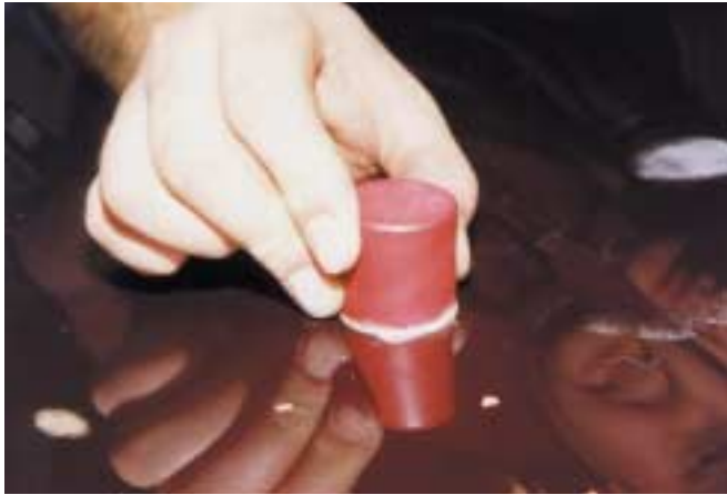
FIGURE 28-19 Here a detail technician is dry sanding dirt in the paint finish with a detail sanding block and ultrafine sandpaper. Dry sanding will more easily let you see how much you have sanded off.
