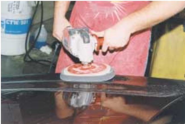
FIGURE 28-35 After buffing with a wool pad, many detail technicians like to machine glaze the paint with a softer foam pad. This will bring out more of the paint shine or gloss.
