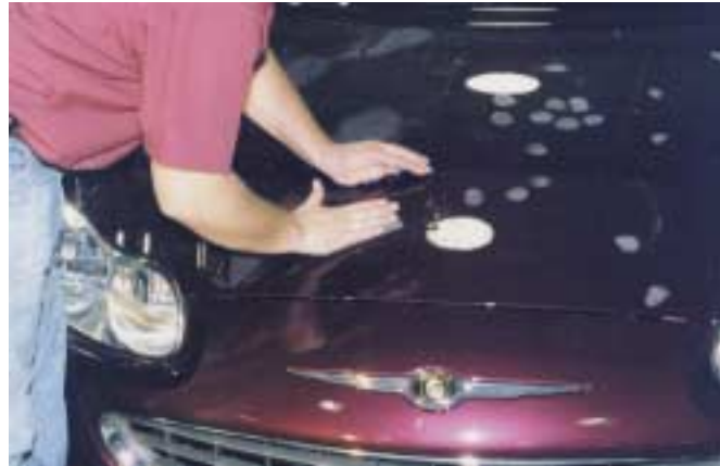
FIGURE 28-21 After dry sanding dirt nibs, wet sand them with #1500 grit sandpaper and water. Wet sand the scratches left from dry sanding. (Photo courtesy of Norton)
