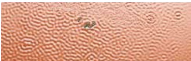
FIGURE 28–10 (A) Lifting and (B) wrinkling are usually caused by incompatible chemicals or using the wrong paint ingredients when mixing.
