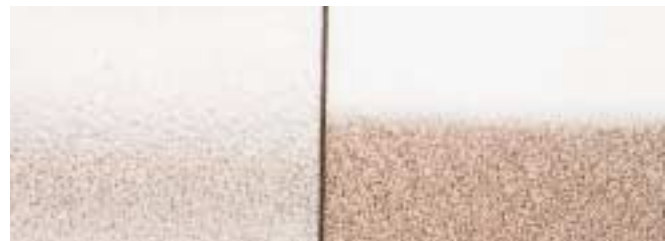
FIGURE 28-1 Note the difference in paint color after this improper panel repair. The metallic paint on the right looks much darker. This could be due to spraying the metallic too wet or to improper tinting.
