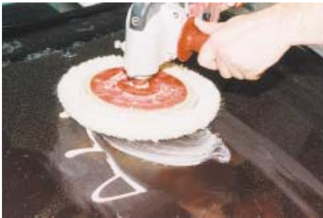
FIGURE 28-32 Before hitting the trigger, spread compound over the area with a pad. This will keep the compound from spraying off the pad.
