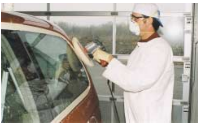
FIGURE 28-33 Normally, you should hold the buffing pad square on the body surface to avoid cutting too deeply into the clearcoat.
