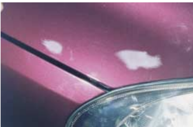
FIGURE 28-20 Only sand enough to knock off the dirt nib. This will dull the finish. (Photo courtesy of Norton)
