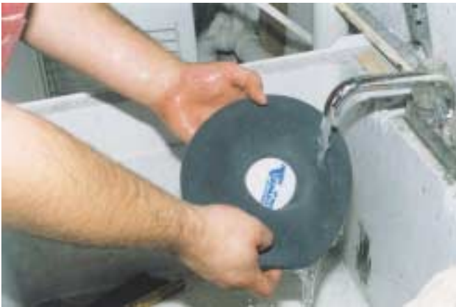
FIGURE 28-27 Your buffing pad should be clean before using it on any vehicle. (A) This technician is using a spur tool to clean and fluff a wool buffing pad. (B) Foam pads should be washed and wetted before use.
