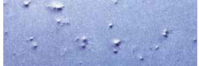
B Dirt in the finish results from larger pieces of lint and larger flakes of dust. This is a highly magnified view.
