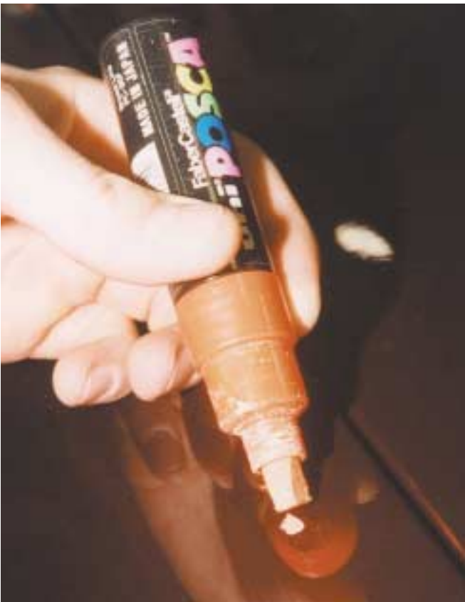
FIGURE 28-17 Use only a paint-safe marker to identify surface imperfections.
