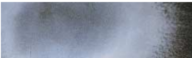
FIGURE 28-7 Blushing is a whitish blotch in paint, normally due to moisture buildup on the painted surface.
