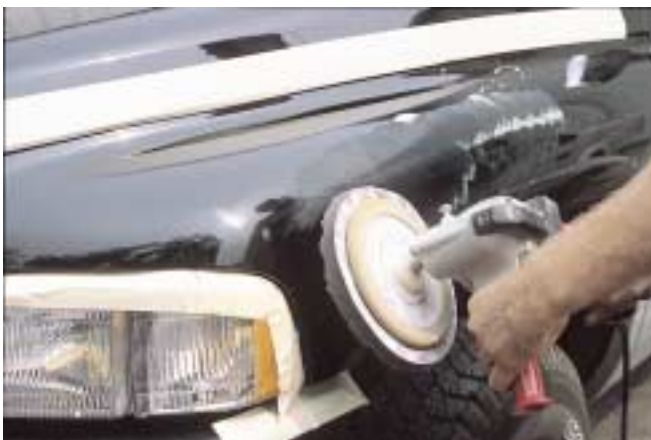
FIGURE 28-36 Note how the plastic headlight lens, plastic parts on the bumper, and sharp body contours have been protected with masking tape.
