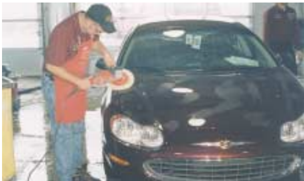
FIGURE 28-30 Buff a panel in passes, just as you would paint it. Move the buffer back and forth in long passes so you can keep track of the amount of paint thickness removal.
