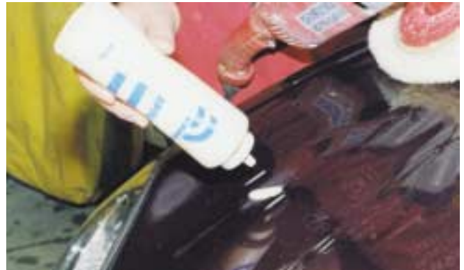
FIGURE 28-31 Only apply enough compound to buff a small area at a time.
