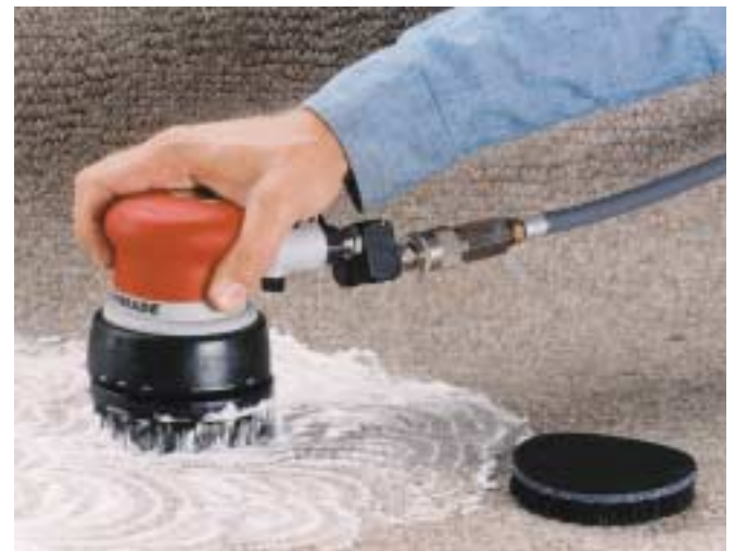
FIGURE 28-37 Here a detail technician is using an air-powered scrubber to clean bloodstains out of carpeting. (Dynabrade Inc.)
