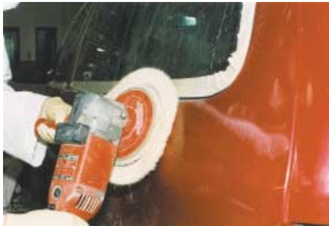
FIGURE 28-34 Be careful when buffing next to the edges of panels. The buffing pad can catch on sharp edges and damage paint or trim pieces.
